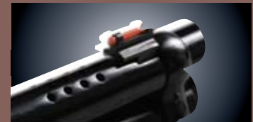
■ Ported barrel of the new Model 92 Carbine .454 Casull.
