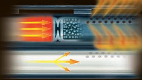
» **Chrome-Plated Chambers and Bores** – a feature on all Reserve models, they maximize corrosion resistance, and at the same time minimize shot/wad friction while traveling the length of the bore.
