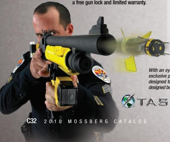
With an eye to innovation, Mossberg is partnering with companies like TASER International to develop exclusive products like the X12 shotgun, a less-lethal-only variant of the Mossberg 500®. The X12 was designed to fire the fully self-contained XREP (eXtended Range Electronic Projectile) shell, while its specially-designed bolt head prevents the accidental chambering or firing of standard ammunition (patent pending).
