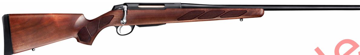
TIKKA T3 HUNTER based on a two locking lug T3 action. Bolt features springloaded plunger ejector and it can be easily stripped down for maintenance. Bolt is made of stainless steel.
