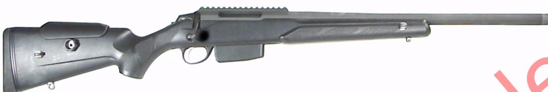
TIKKA T3 TACTICAL based on a two locking lug T3 action. Bolt features springloaded plunger ejector and it can be easily stripped down for maintenance. Bolt is made of stainless steel and tefloncoated. Other outer steel parts are manganese phosphatized.
